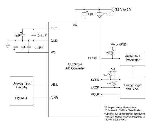
Figure 2. CS5343/4 Typical Connection Diagram
