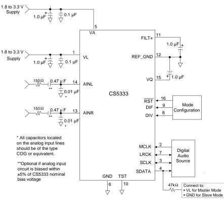
Figure 1. CS5333 Typical Connection Diagram
