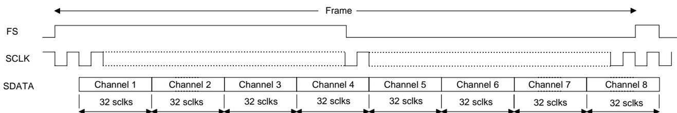
**Figure 3. CS5368/66/64 TDM Mode as System Clock Master**
