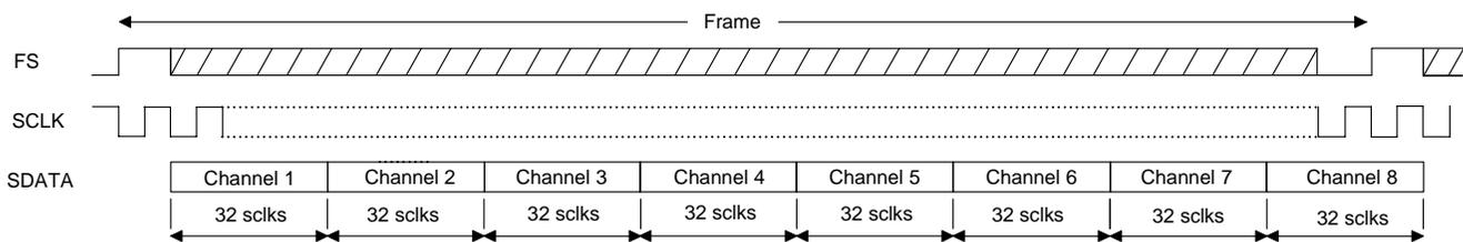
**Figure 2. CS5368/66/64 TDM Mode as System Clock Slave**
