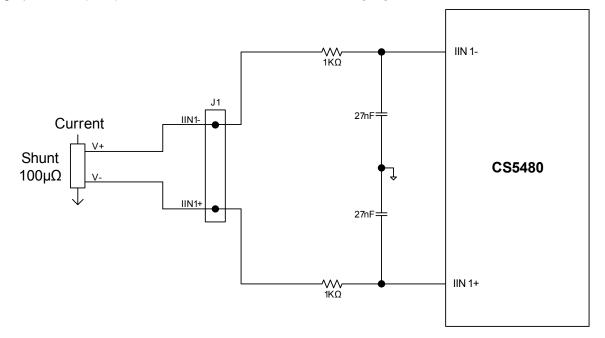
Figure 10. Connection between Shunt and CS5480
