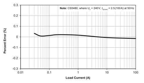
Figure 9. I<sub>RMS</sub> Load Current Performance
