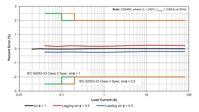
Figure 4. Reactive Energy Load Performance vs IEC 62053-23 Class 2 Standard
