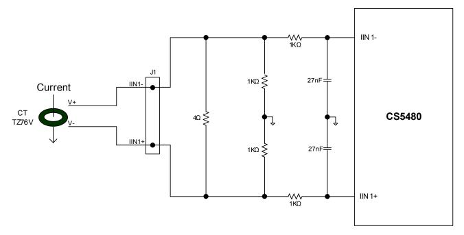
Figure 6. Connection between Current Transformer CT and CS5480
