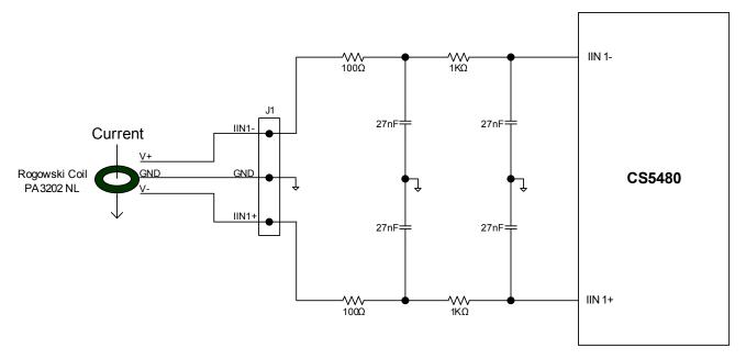
Figure 2. Connection between Rogowski Coil and CS5480
