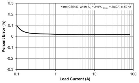
Figure 5. I<sub>RMS</sub> Load Current Performance
