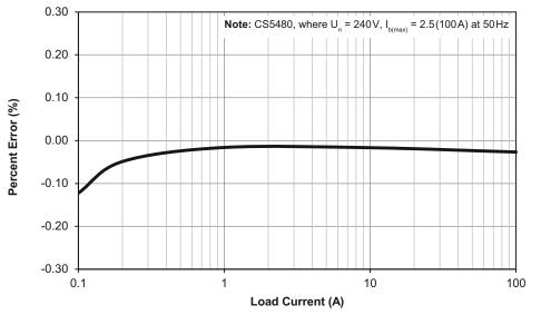
Figure 13. I<sub>RMS</sub> Load Current Performance
