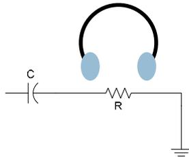
**Figure 7 High-pass Network Formed by a.c. Coupling**
