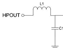
**Figure 2 Low-pass PWM Filter**
