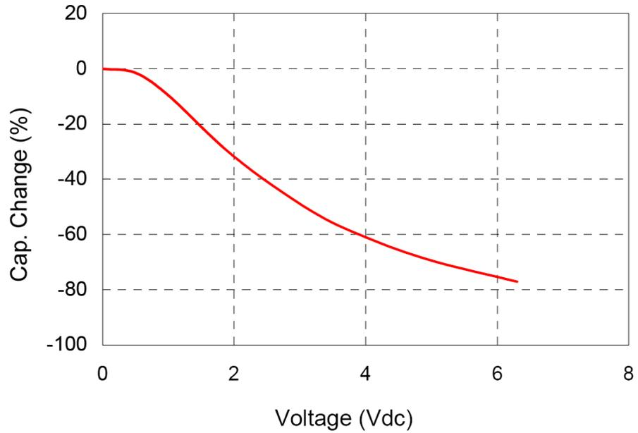
Figure 2 Capacitor DC Co-efficient Graph (GRM155R60J225ME15\_EIA)
