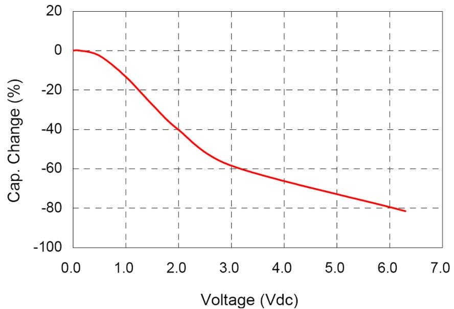
Figure 3 Capacitor DC Co-efficient Graph (GRM155R60J475M\_EIA)
