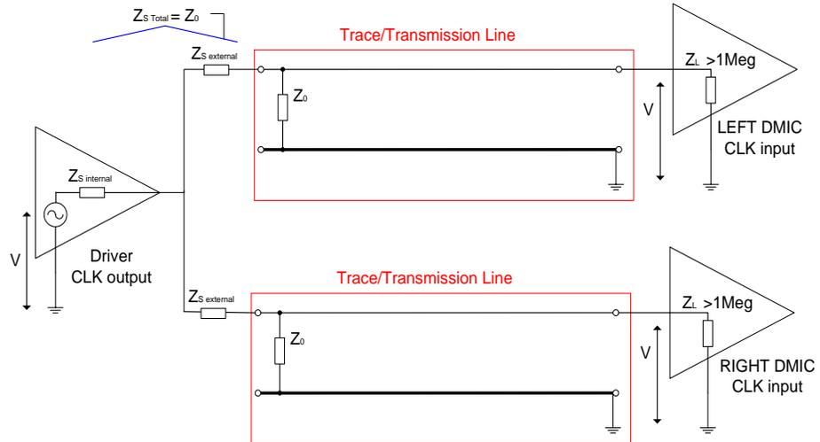
**Figure 6 Source Termination for Stereo Microphone Interface**
