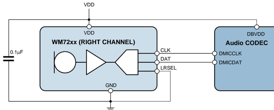
**Figure 2 Mono Digital Microphone Interface**
