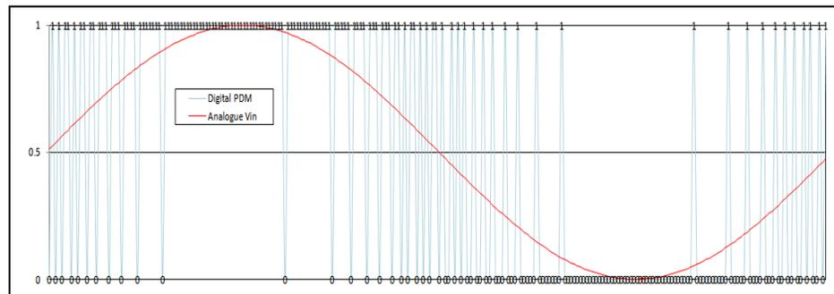
**Figure 1 PDM Representation of Analogue Input Sine Wave**
