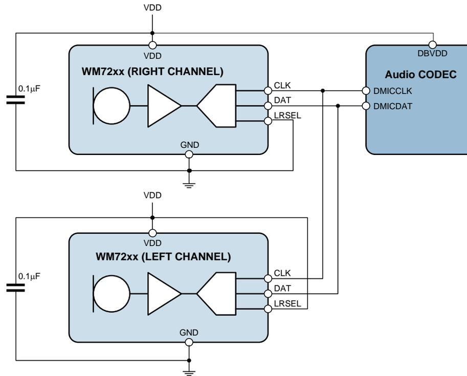
**Figure 3 Stereo Digital Microphone Interface**
