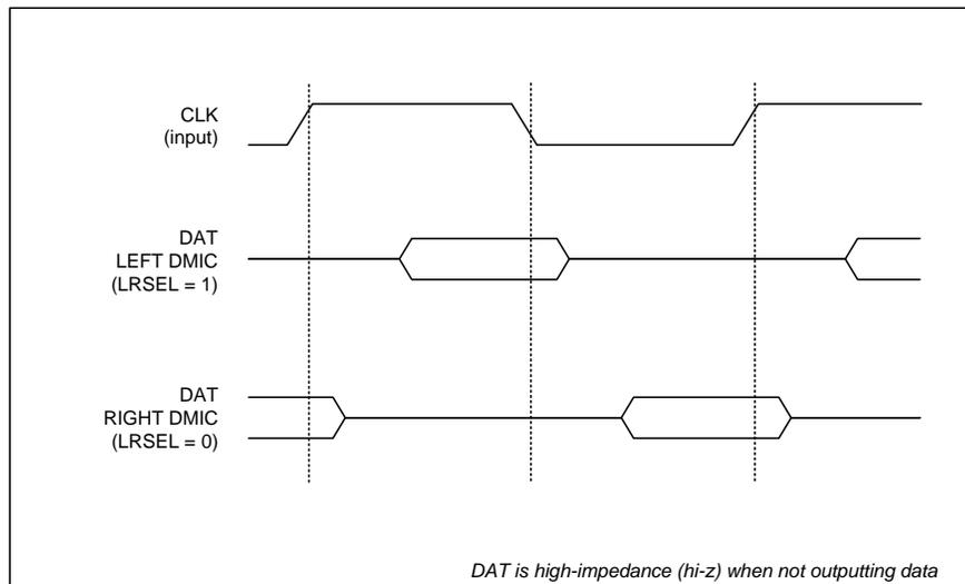
**Figure 4 Output Data on Stereo DMIC Configuration**
