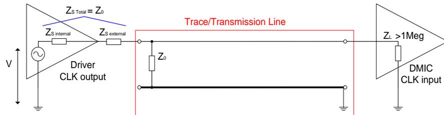
**Figure 5 Source Termination of Single DMIC Circuit**
