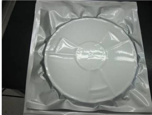
**Figure 2 Air-Leakage of Microphone Drybag**
