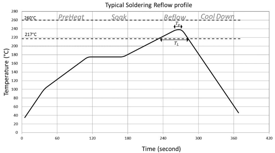
**Figure 6 Typical Solder Reflow Profile**
