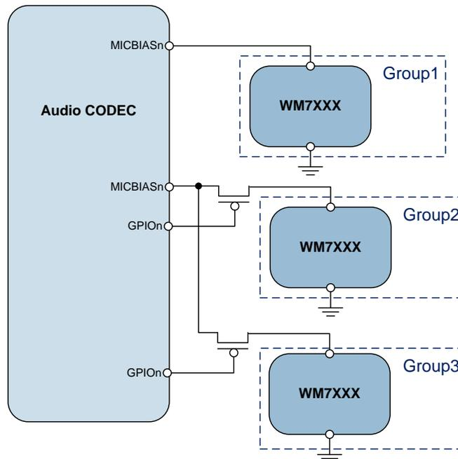
**Figure 4 Power Gating using Discrete PMOS Devices**
