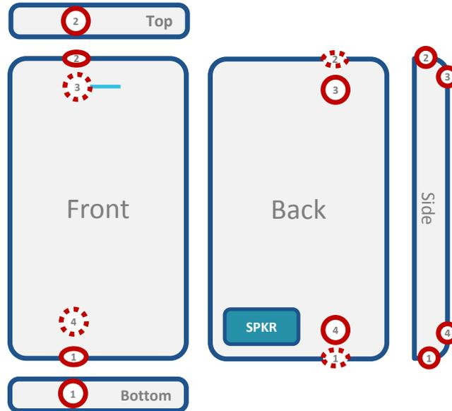
**Figure 1 Example Microphone Placement in a Mobile Phone**
