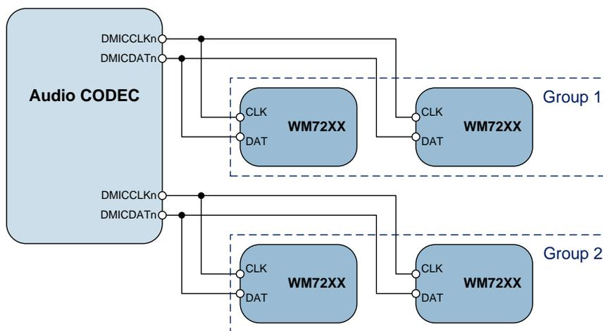
**Figure 7 Clock Gating Using a Standard Digital Microphone Circuit**
