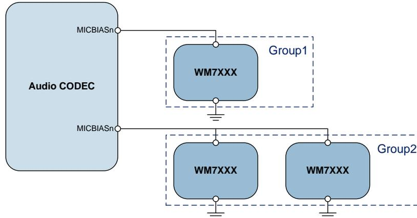
**Figure 3 Power Gating using Independently Enabled MICBIAS Outputs**
