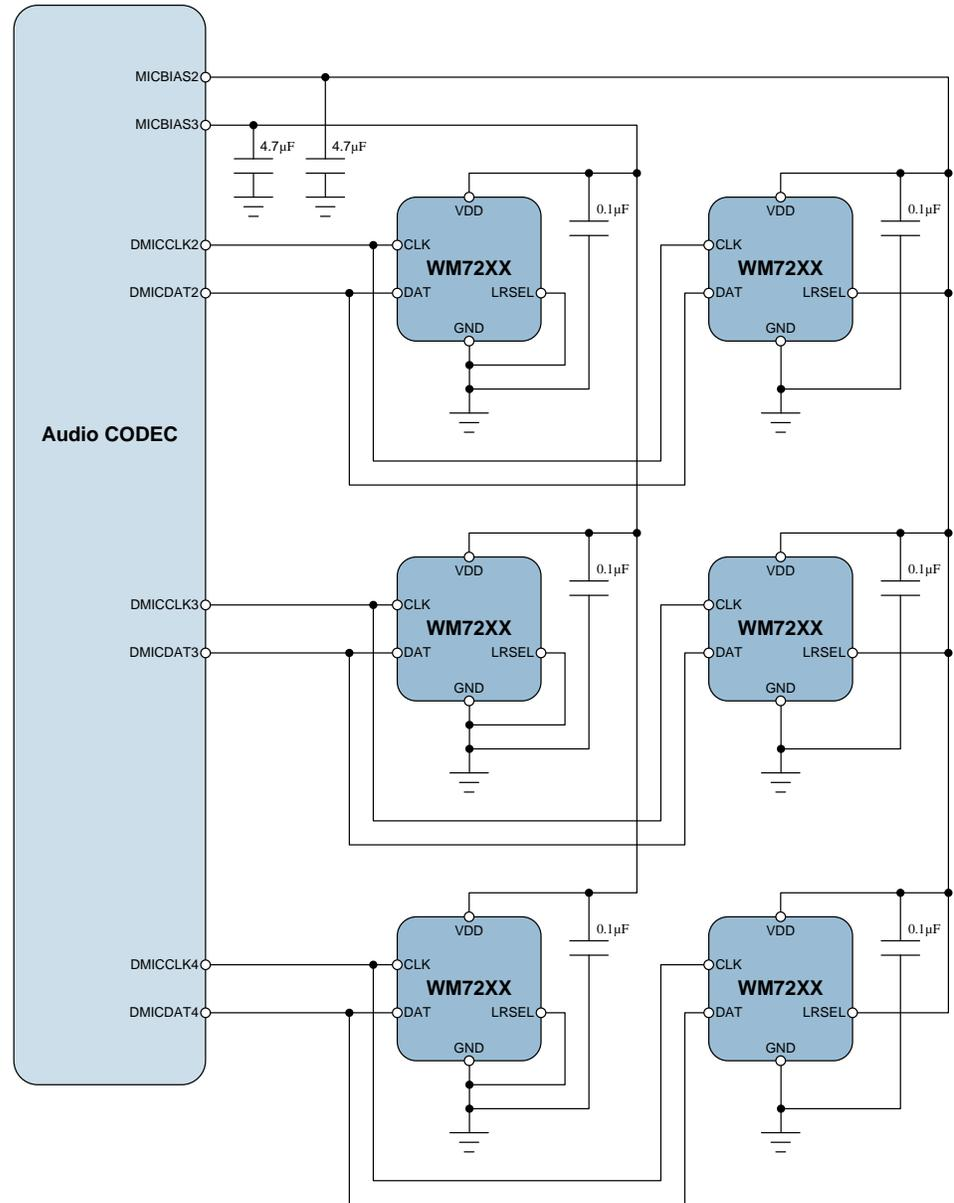
**Figure 8 Digital Microphone Array with Combined Supply and Clock Gating**
