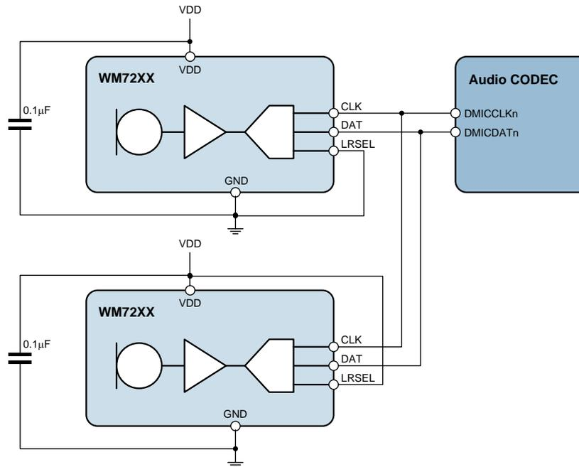
**Figure 6 Example Digital Microphone Schematic**
