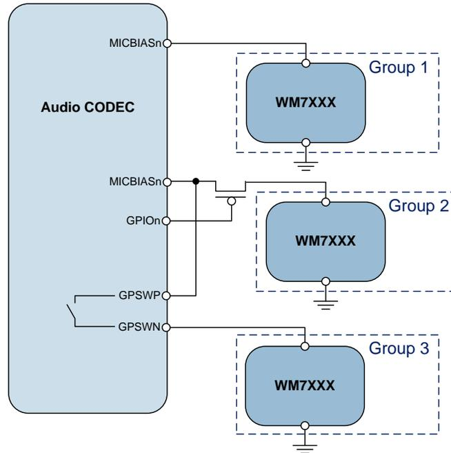
**Figure 5 Power Gating using the General Purpose Switch**
