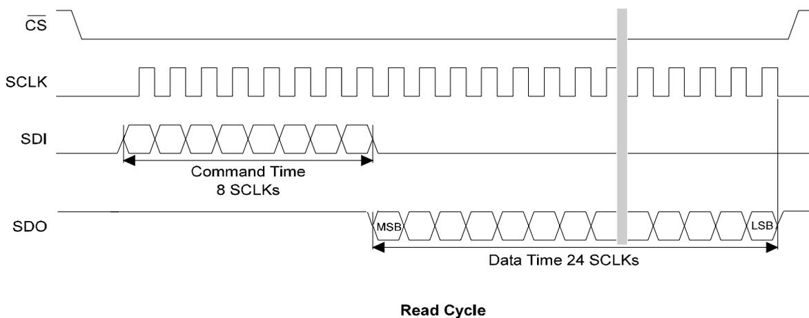
**Figure 4. Read-Cycle Timing**
