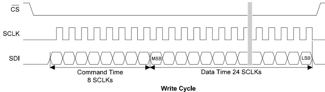
**Figure 3. Write-Cycle Timing**
