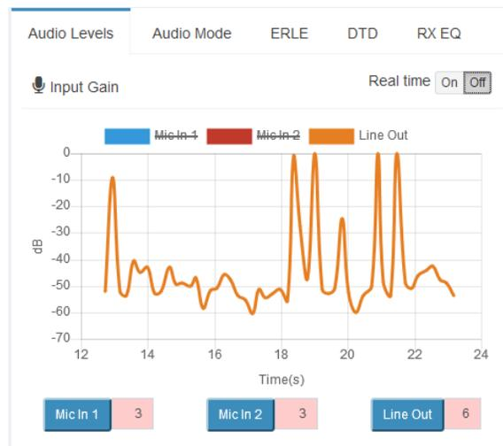
**Figure 9 Graph – Audio Level with Clipping**
