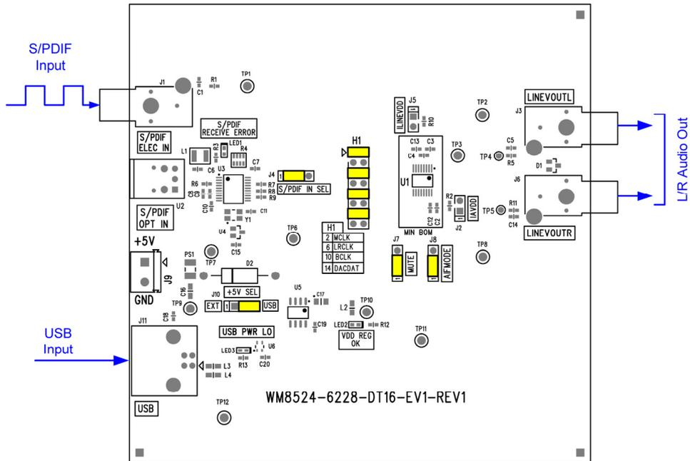
Figure 3 Board Configuration
