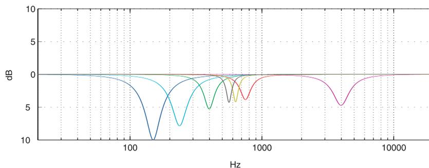
7-band equalizer characteristics after calibration.
