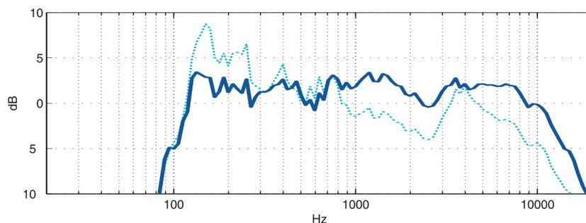
Dotted line indicates performance before calibration. Solid line indicates performance after calibration.
