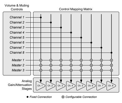
Figure 5. CS3308 Control Mapping Matrix
