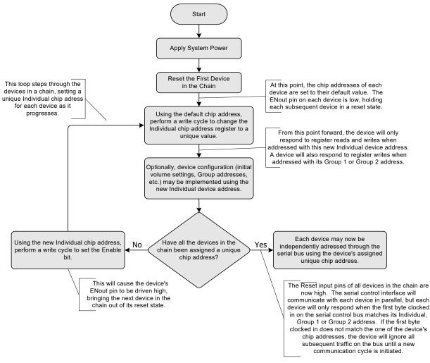
Figure 10. Individual Device Address Configuration Process
