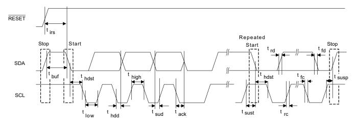
Figure 1. Control Port Timing - I<sup>2</sup>C Format
