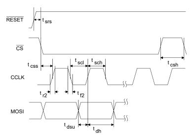
Figure 2. Control Port Timing - SPI Format
