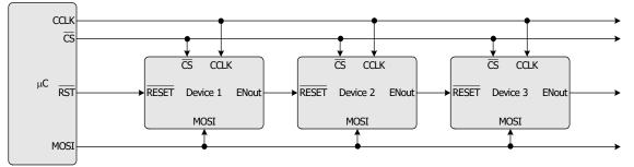
Figure 9. SPI Serial Control Connections
