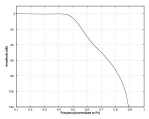
Figure 40. Quad-Speed (slow) Stopband Rejection
