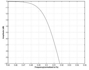
Figure 26. Single-Speed (slow) Transition Band (detail)
