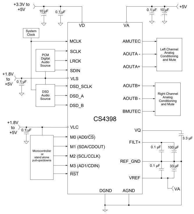
Figure 10. Typical Connection Diagram
