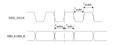
Figure 6. Direct Stream Digital - Serial Audio Input Timing
