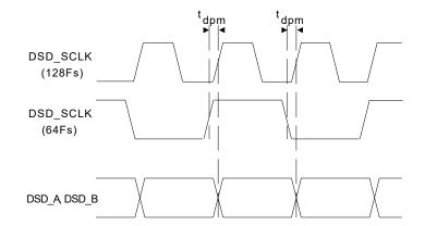
Figure 7. Direct Stream Digital - Serial Audio Input Timing for Phase Modulation Mode
