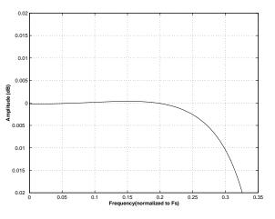
Figure 35. Double-Speed (slow) Passband Ripple
