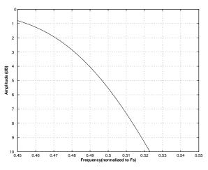
Figure 42. Quad-Speed (slow) Transition Band (detail)
