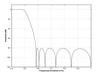
Figure 28. Double-Speed (fast) Stopband Rejection
