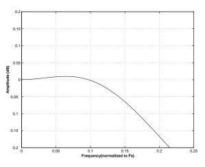
Figure 39. Quad-Speed (fast) Passband Ripple
