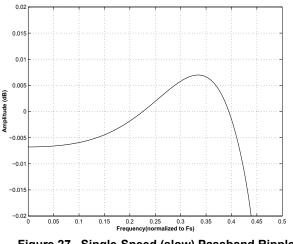
Figure 27. Single-Speed (slow) Passband Ripple
