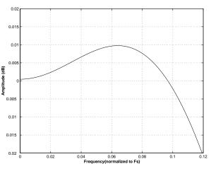
Figure 43. Quad-Speed (slow) Passband Ripple
