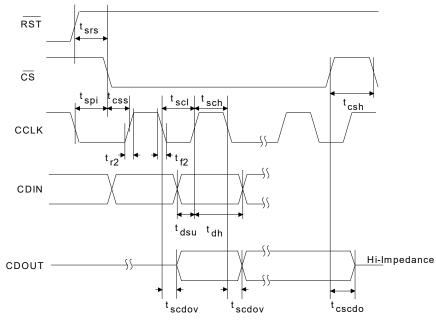
Figure 9. Control Port Timing - SPI Format (Read/Write)
