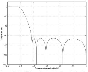
Figure 24. Single-Speed (slow) Stopband Rejection
