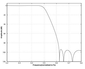
Figure 37. Quad-Speed (fast) Transition Band
