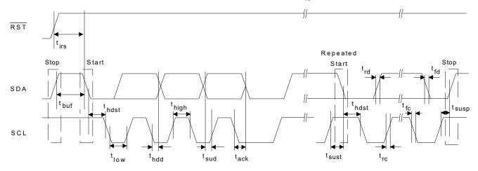
Figure 8. Control Port Timing - I<sup>2</sup>C Format
