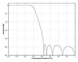
Figure 36. Quad-Speed (fast) Stopband Rejection
