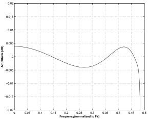
Figure 23. Single-Speed (fast) Passband Ripple
