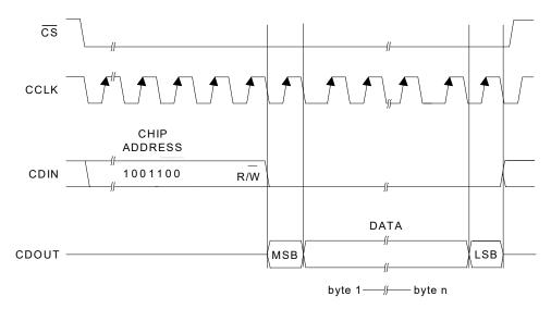
Figure 16. Control Port Timing, SPI Format (Read)
