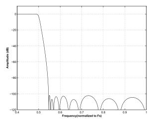
Figure 20. Single-Speed (fast) Stopband Rejection
