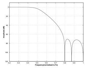
Figure 32. Double-Speed (slow) Stopband Rejection
