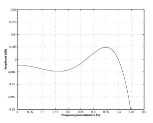
Figure 31. Double-Speed (fast) Passband Ripple
