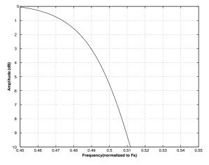
Figure 38. Quad-Speed (fast) Transition Band (detail)
