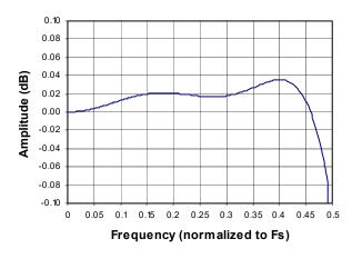
Figure 20. Single-Speed Passband Ripple
