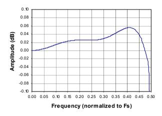
Figure 24. Double-Speed Passband Ripple
