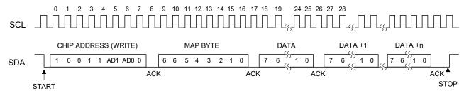
Figure 15. Control Port Timing, I2C Write
