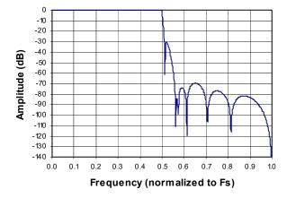
Figure 21. Double-Speed Stopband Rejection
