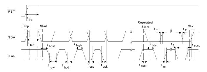
Figure 5. Control Port Timing - I<sup>2</sup>C Format
