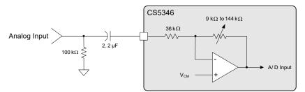
Figure 11. 1 V<sub>RMS</sub> Input Circuit
