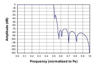
Figure 17. Single-Speed Stopband Rejection
