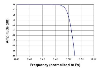
Figure 23. Double-Speed Transition Band (Detail)
