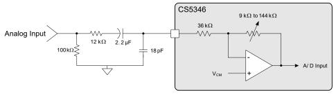
Figure 13. 2 V<sub>RMS</sub> Input Circuit
