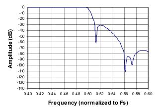
Figure 22. Double-Speed Stopband Rejection
