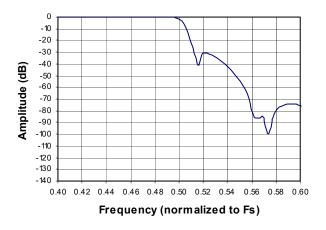
Figure 18. Single-Speed Stopband Rejection
