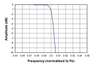
Figure 19. Single-Speed Transition Band (Detail)
