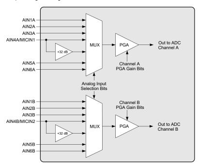
Figure 9. Analog Input Architecture
