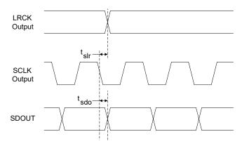
Figure 2. Slave Mode Serial Audio Port Timing
