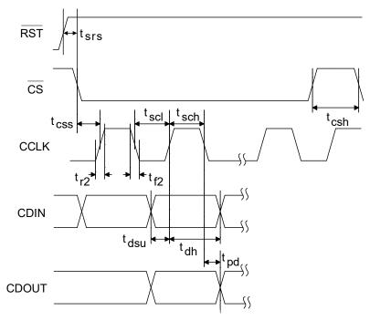
Figure 6. Control Port Timing - SPI Format
