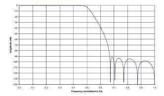
Figure 5. Double-Speed Mode Stopband Rejection
