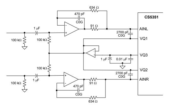
Figure 24. CS5351 Recommended Analog Input Buffer
