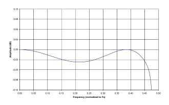
Figure 4. Single-Speed Mode Passband Ripple
