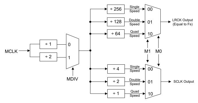
Figure 23. CS5351 Master Mode Clocking
