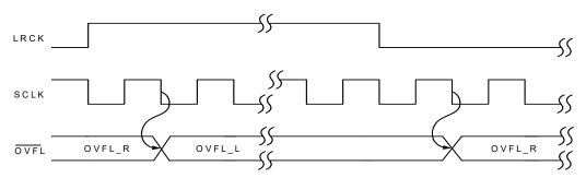
Figure 21. OVFL Output Timing, Left-Justified Format
