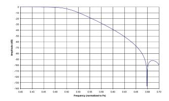
Figure 6. Double-Speed Mode Transition Band
