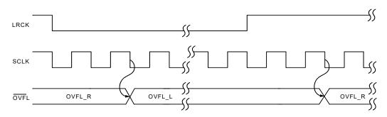
Figure 20. OVFL Output Timing, I<sup>2</sup>S Format
