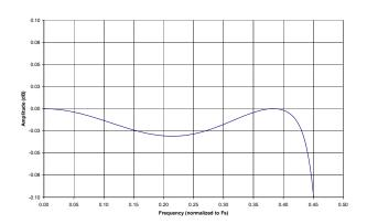
Figure 8. Double-Speed Mode Passband Ripple
