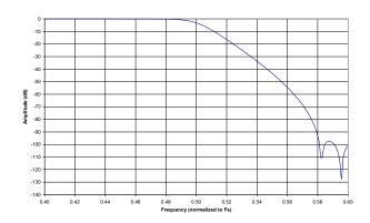
Figure 2. Single-Speed Mode Transition Band
