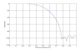
Figure 9. Quad-Speed Mode Stopband Rejection
