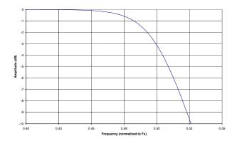
Figure 7. Double-Speed Mode Transition Band (Detail)
