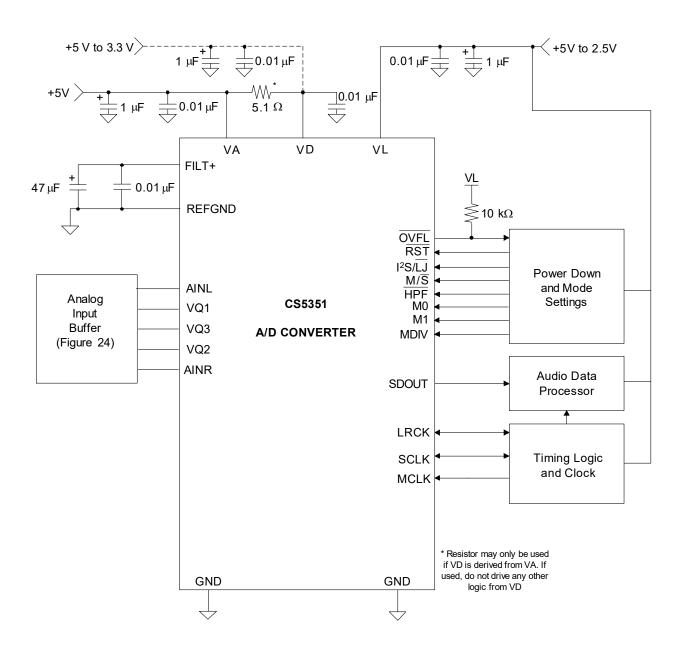
Figure 22. Typical Connection Diagram
