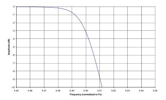
Figure 3. Single-Speed Mode Transition Band (Detail)
