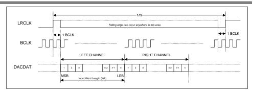
Figure 21 DSP Mode Audio Interface (mode A, AIF\_LRCLK\_INV=0, Slave)
