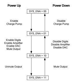
Figure 23 SYS\_ENA[1:0] Power Up and Down Sequences
