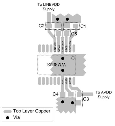
Figure 38 Recommended PCB Layout
