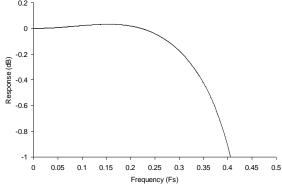
Figure 29 DAC Digital Filter Frequency Response
