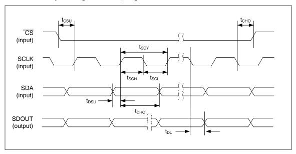
Figure 5 Control Interface Timing - SPI Control Mode (Read Cycle)
