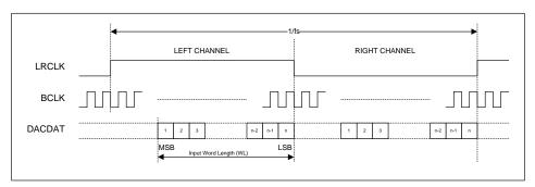
Figure 16 Right Justified Audio Interface (assuming n-bit word length)
