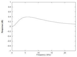
Figure 35 De-Emphasis Frequency Response (48kHz)
