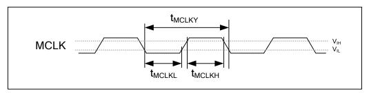
Figure 1 System Clock Timing Requirements
