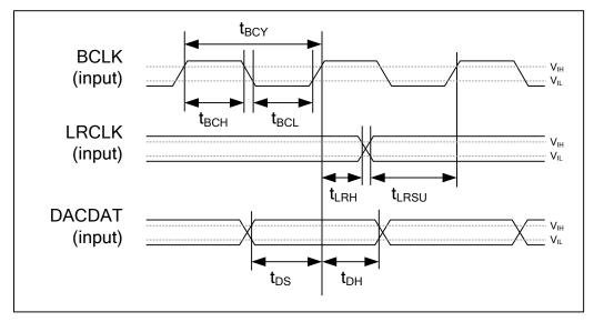
Figure 3 Digital Audio Data Timing - Slave Mode
