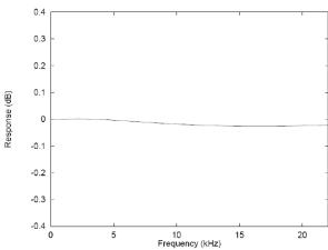
Figure 33 De-Emphasis Frequency Response (44.1kHz)
