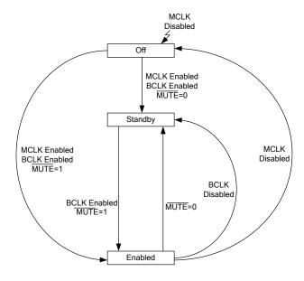
Figure 25 Hardware Power Sequence Diagram
