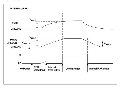
Figure 7 Typical Power Timing Requirements
