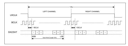
Figure 18 I<sup>2</sup>S Justified Audio Interface (assuming n-bit word length)
