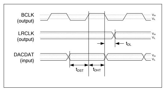
Figure 2 Master Mode Digital Audio Data Timing
