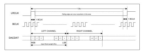
Figure 22 DSP Mode Audio Interface (mode B, AIF\_LRCLK\_INV=1, Slave)
