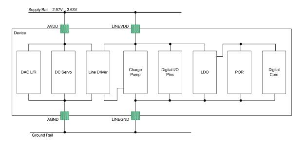
Figure 26 Power Domain Diagram
