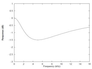
Figure 31 De-Emphasis Frequency Response (32kHz)
