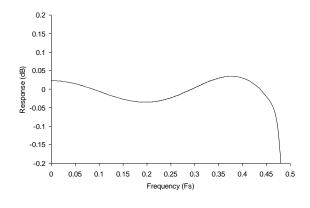
Figure 27 DAC Digital Filter Frequency Response
