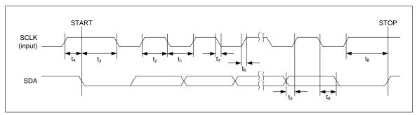
Figure 4 Control Interface Timing – I<sup>2</sup>C Control Mode
