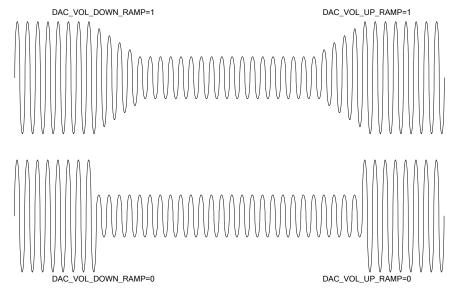
Figure 24 Volume Ramp Functionality
