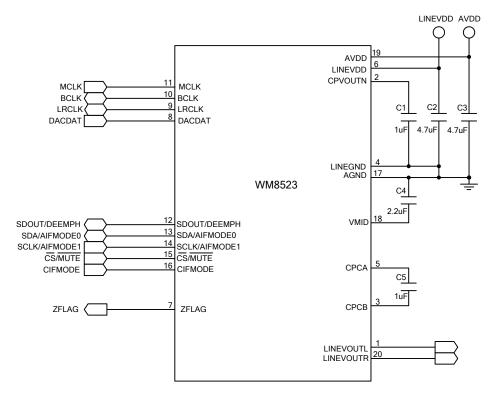
Figure 37 Recommended External Components
