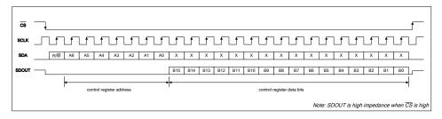
Figure 13 SPI Control Interface - read operation
