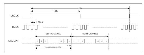
Figure 19 DSP Mode Audio Interface (mode A, AIF\_LRCLK\_INV=0, Master)
