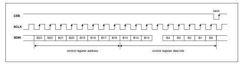
Figure 34 3-Wire Serial Control Interface
