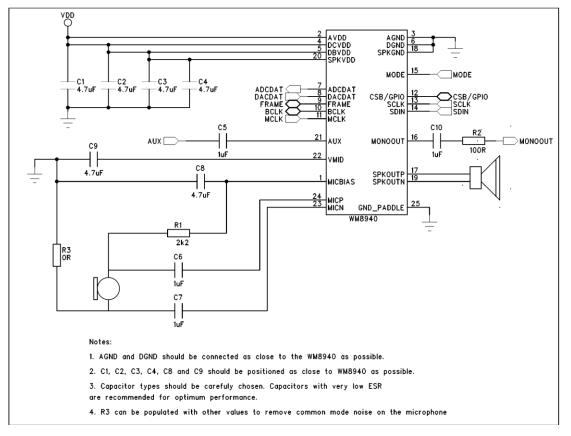
Figure 49 Recommended External Components
