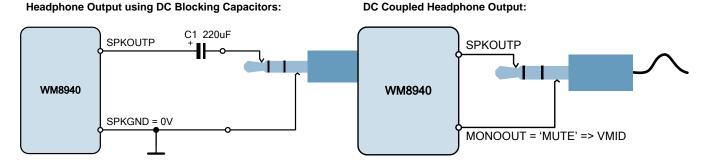
Figure 23 Recommended Headphone Output Configurations
