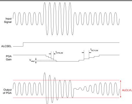
Figure 13 ALC Limiter Mode Operation
