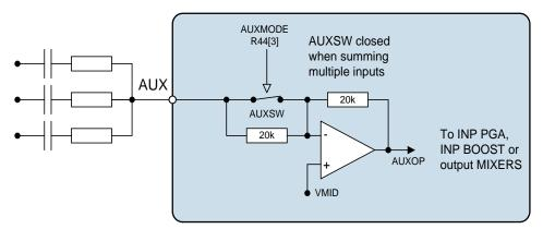
Figure 7 Auxiliary Input Circuit
