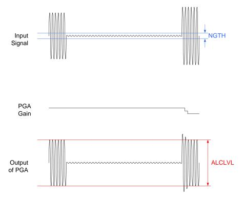
Figure 18 Noise Gate Operation
