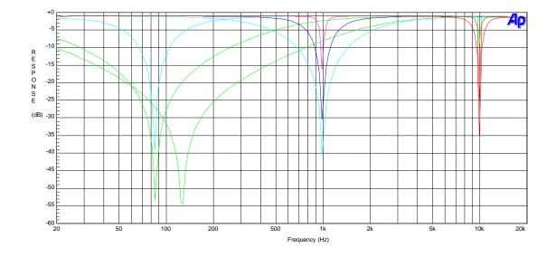
Figure 46 ADC Notch Filter Responses (48kHz); fc=100Hz, 1kHz, 10kHz; fb = 100Hz, 600Hz, 2kHz
