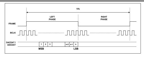
Figure 26 Right Justified Audio Interface (assuming n-bit word length)
