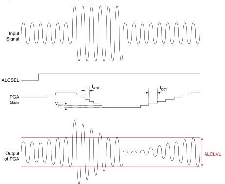
Figure 12 ALC Normal Mode Operation
