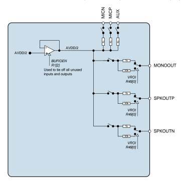
Figure 21 Unused Input/Output Pin Tie-off Buffers
