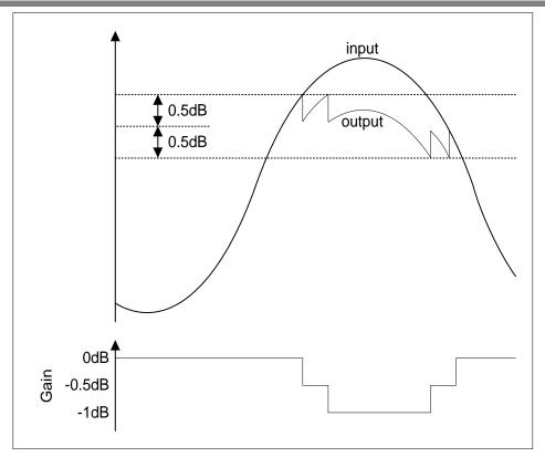
Figure 20 DAC Digital Limiter Operation
