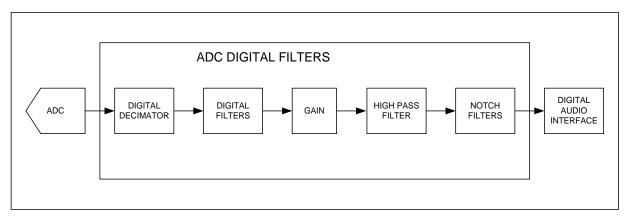
Figure 10 ADC Digital Filter Path
