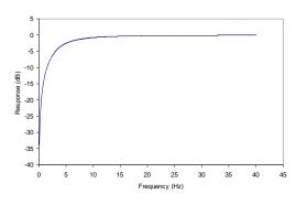
Figure 42 ADC High pass Filter Response, HPFAPP=0
