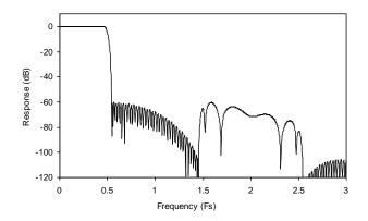
Figure 40 ADC Digital Filter Frequency Response
