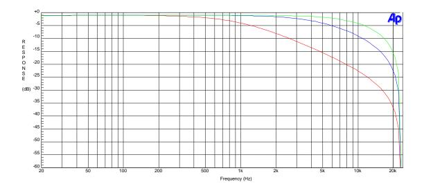
Figure 47 ADC Low Pass Filter Responses (48kHz); fc= 1kHz, 5kHz, 10kHz
