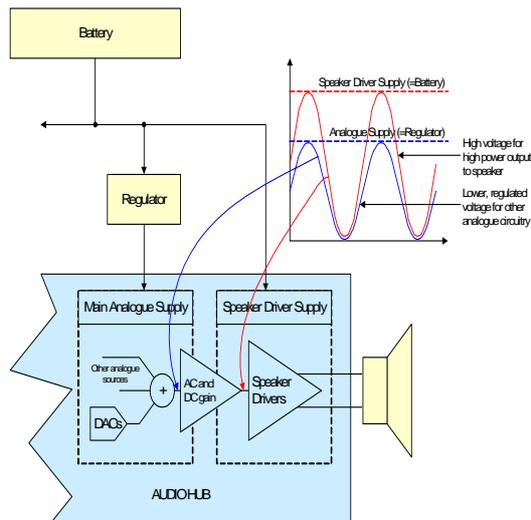
**Figure 7: Internal Signal Boosting to Maximise Speaker Volume**
