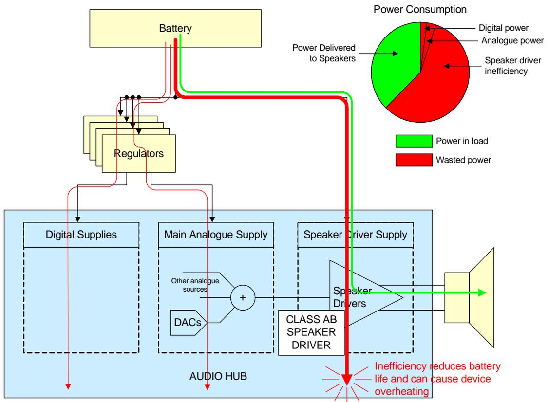
**Figure 8: Class AB Speaker Drivers: Reduced Battery Life and Potential Overheating**
