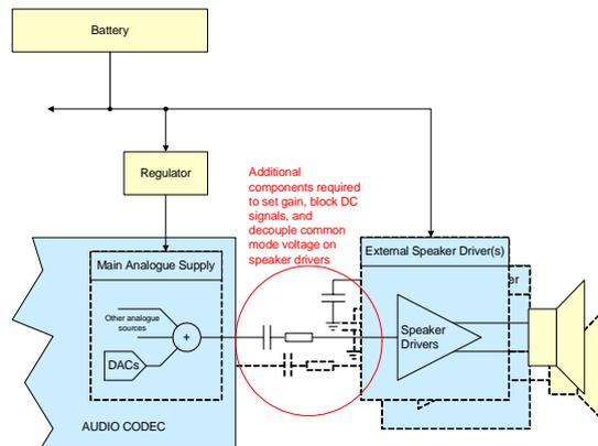
**Figure 6: External Speaker Drivers: Increased Component Count**
