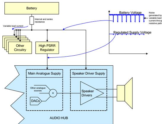
**Figure 3: Typical Power Supply Arrangement in Portable Multimedia Applications**
