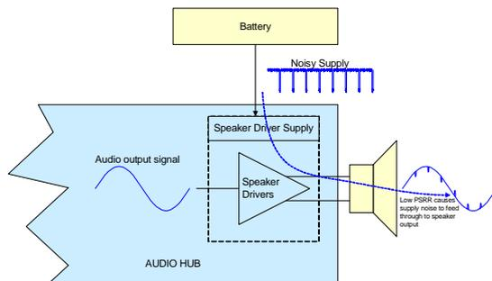
**Figure 4: Effects of Low PSRR on Speaker Output**
