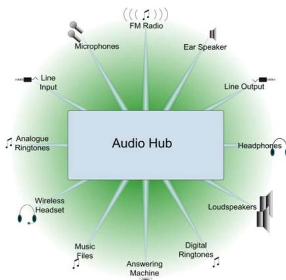
The audio hub must be capable of interfacing analogue signals of varying magnitudes, source impedances, DC offsets and bandwidths, such as FM receivers, microphones, send/receive voice data, ringtones or hi-fi line input. Flexible input configurations can provide support for these diverse signal characteristics in different system architectures while minimising pin count, saving space and reducing costs.
