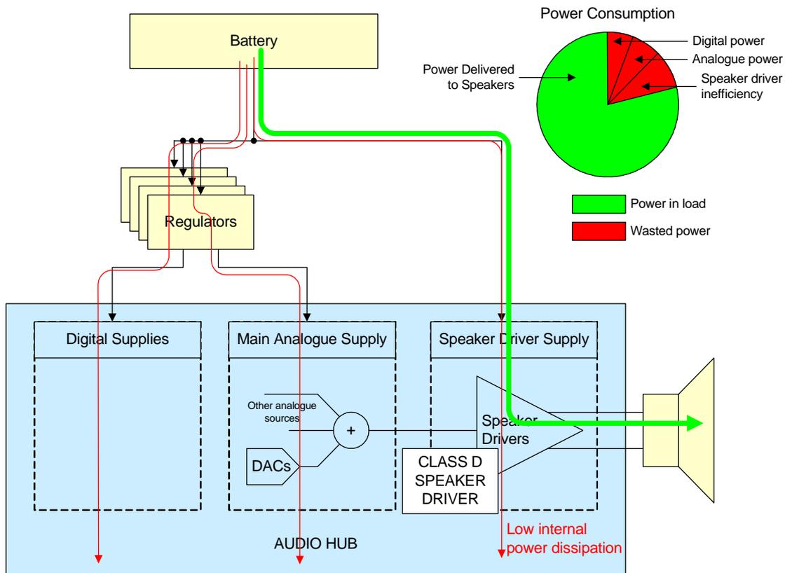
**Figure 9: Class D Speaker Drivers: Increased Efficiency**
