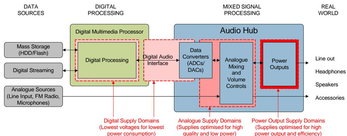
**Figure 1: Typical Portable Multimedia System**
