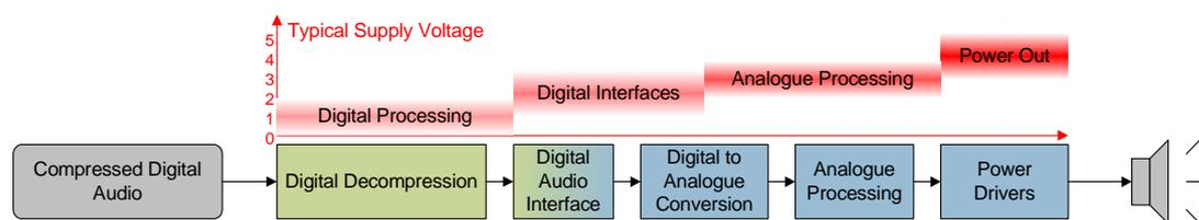
**Figure 2: Digital Audio Playback Signal Chain**
