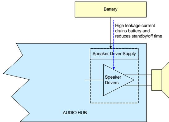
**Figure 5: Leakage Current in Speaker Drivers**
