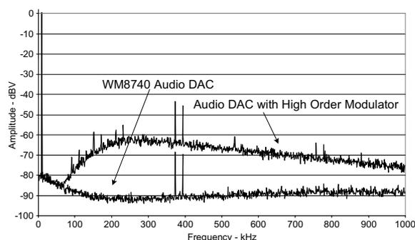
Figure 10. Out-of-band DAC spectra (from [17]).
