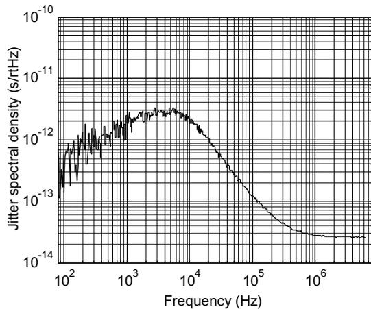
Figure 4. Idealized PLL jitter spectrum.
