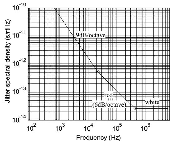
Figure 3. Asymptotes of oscillator jitter spectra.
